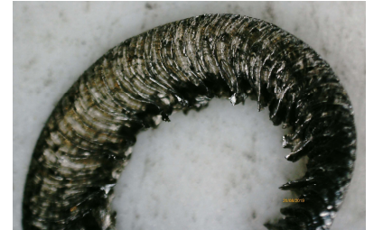
Lamellar chip flow, MR YG214 SS304
